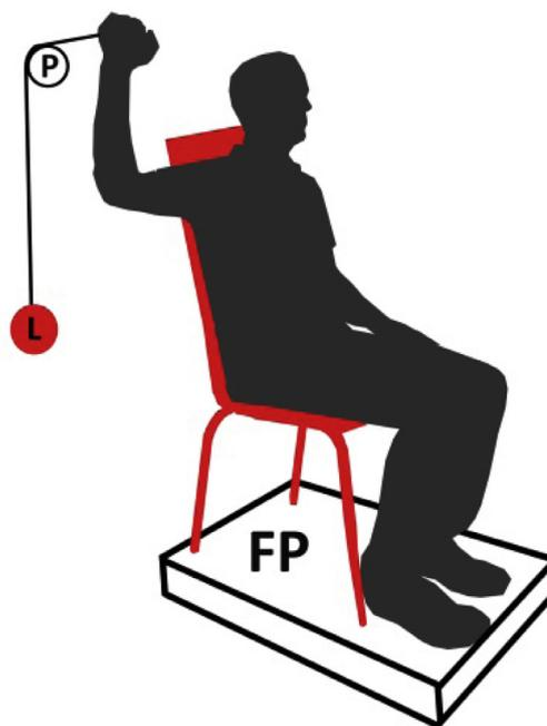
**Fig. 1.** Experimental set-up illustrating a subject sitting on chair resting on a force plate (FP). The load ( $L$ ) is attached to the hand by a rope to create a horizontal force through a pulley ( $P$ ) system. The upper limb joint positions and the applied load were set at 90°.
