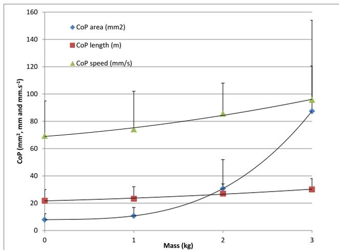
Fig. 3. Center of pressure (CoP) area, length and speed for four shoulder loads. The vertical bars represent the upper values of their respective standard deviation.
