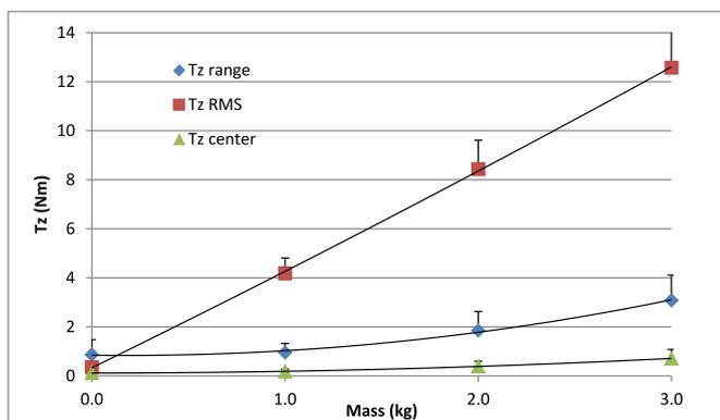
Fig. 4. Free moment (Tz) range, rms and centered rms value for four shoulder loads. The vertical bars represent the upper values of their respective standard deviation.
